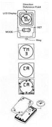
Once calibrated properly, the LCD display will show the direction you are facing while looking through the binocular. The small triangle containing the letter "N" will always point to the north.
